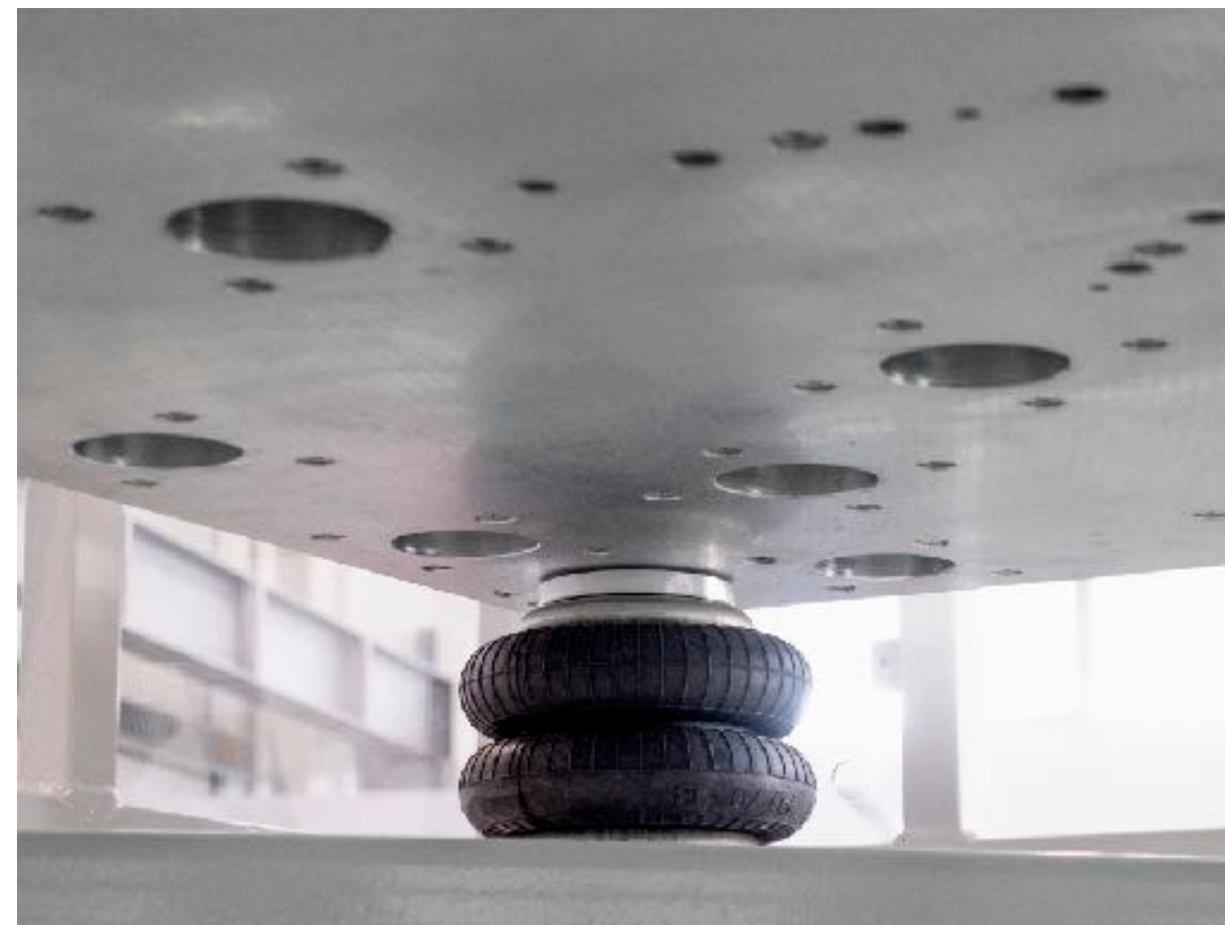
Load support by air springs
