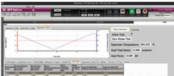
To run a “zero stress” test, simply set the control so that “0” mechanical strain is applied while cycling temperature and monitoring stress.
