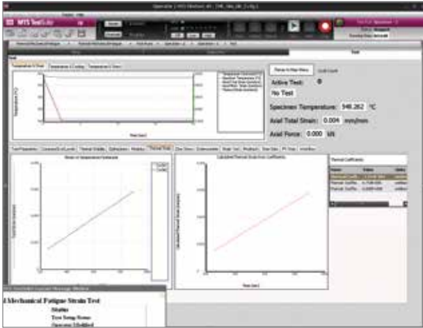
View intuitive graphical depictions of zero load and temperature cycling only to measure the correlation coefficients between expansion and temperature.
