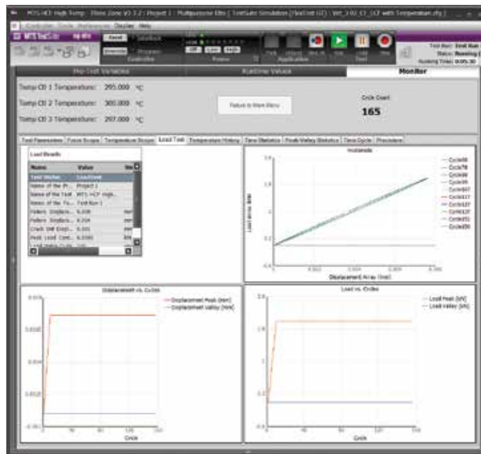
The Runtime View provides a comprehensive view of ADVHCF tests in progress, test setup parameters, load versus displacement, displacement versus cycles, peak valley load versus cycles and much more.
