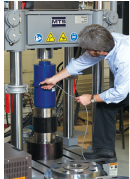
Load Frame Calibration
