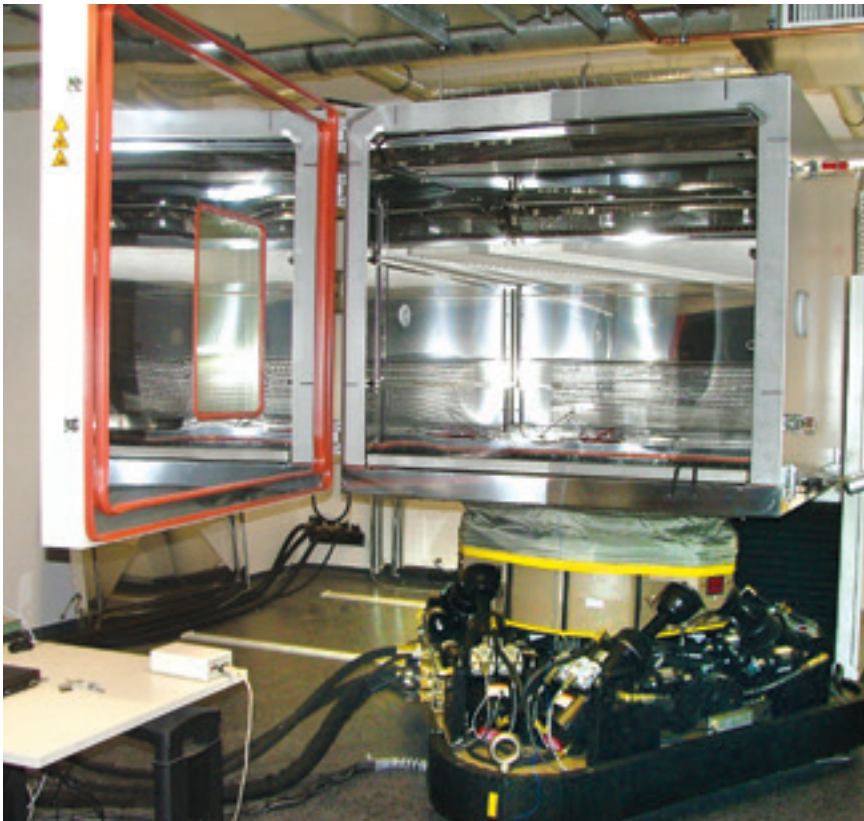
Model 353 MAST system with integrated environmental chamber at PLDS Automotive Test Laboratory in Wetzlar Germany (Photo courtesy of PLDS Germany GmbH)
