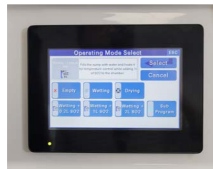
Automatic SO2 Dosing System
