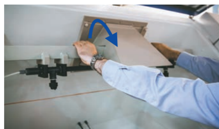
2. The combined air dispersal and oscillating spray bar unit simply lifts out.
