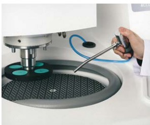
Retractable water hose for easy cleaning
